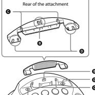
4 Align the projections of the bottom of the attachment (**①**) to the corresponding indentations of the Dock, and push
